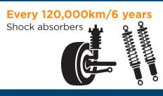
Service items are replaced either by km's or time – whichever comes first. Timeframes are based on normal driving conditions. Adverse driving such as heavy traffic, heavy braking and accelerating will increase replacement frequency.
